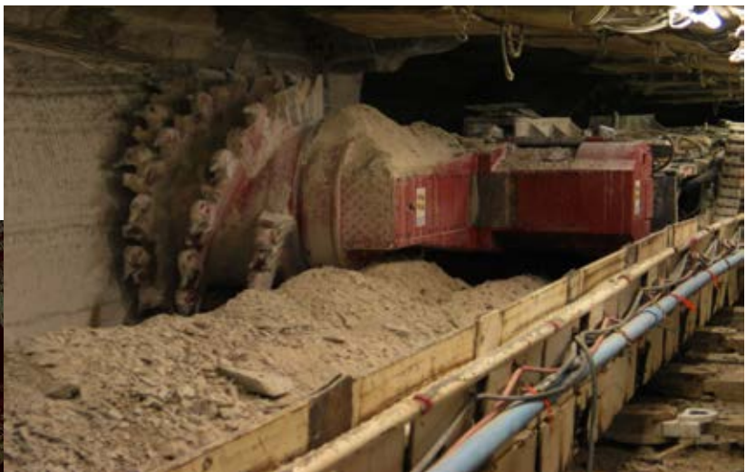
Boring machine (left) and longwall mining machine (right) working trona mines (Wyoming Mining Association)
