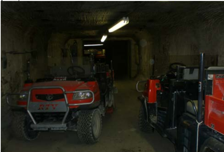
Inside a room-and-pillar trona mine with RTVs, Solvay Chemicals (Toxey/McMillan Design Associates)
